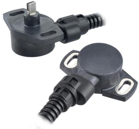
The SRH301 and SRH302 range of shaft-operated Rotary Position Sensors offers the optimal combination of performance, safety and cost. The sensor utilises proven Hall-effect, sensing technology in a low-profile (17.3mm) housing with integral magnet.
